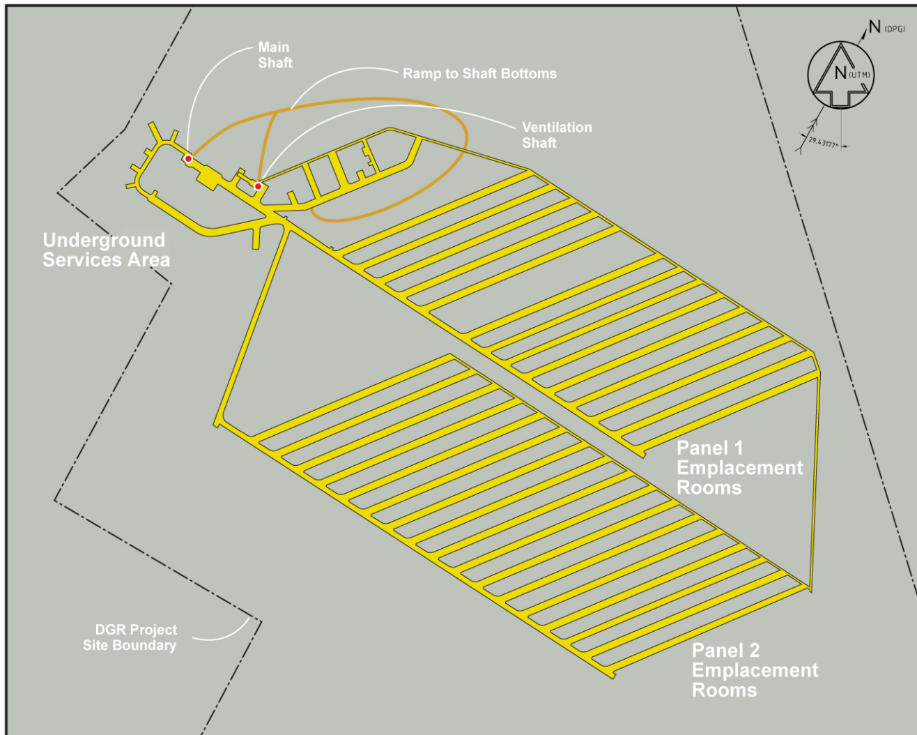
Figure 4.4.2-1: Preliminary Layout of the Underground Repository
